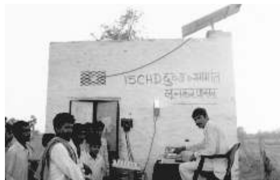
Fig. 5.12: Solar operated electronic milk testing equipment
