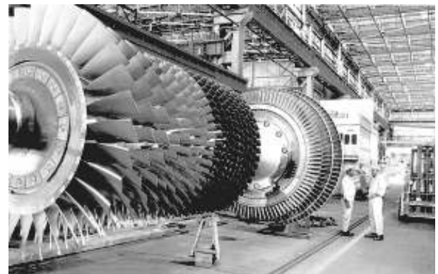
Fig. 6.10: Gas turbine rotor on an assembly bed at BHEL, Hyderabad
